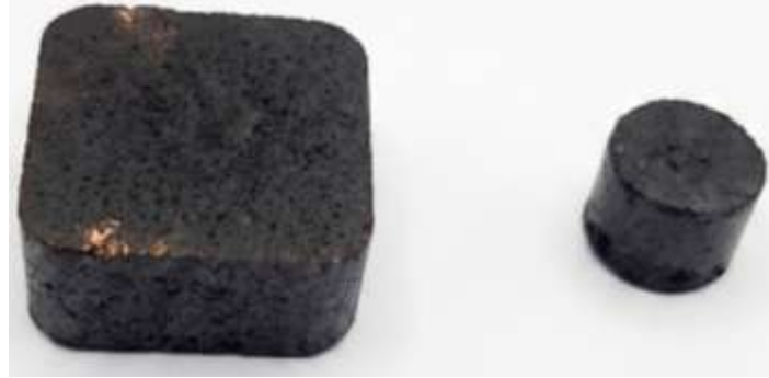
Figure 1. Photograph of the fabricated PPA25 brake pad specimens used in the experimental study
