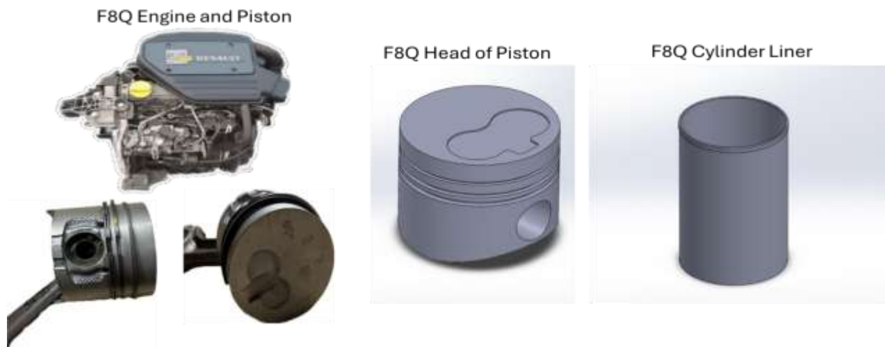
Figure 4. F8Q engine and modeled piston-cylinder liner
