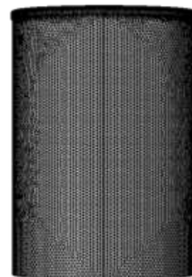
Figure 6. Mesh of cylinder liner
