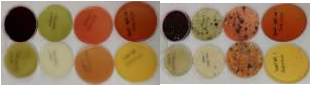
Figure 28. ½ Fresh fruit and vegetable waste and starch + gelatin added oven-dried films
