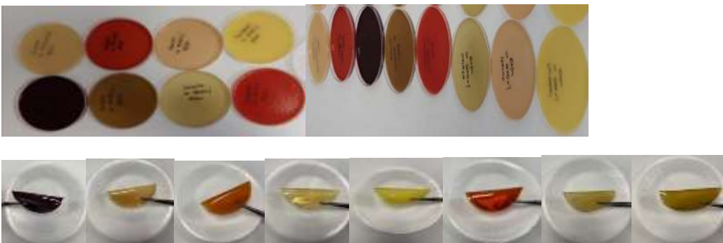
Figure 8. Oven-dried fruit and vegetable wastes and gelatin-added microwave + room-dried films.
