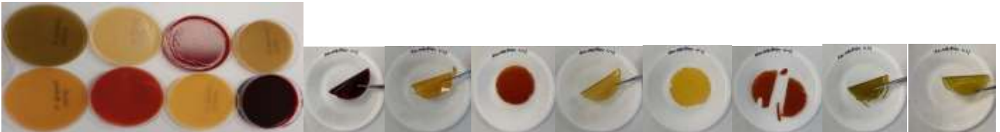
Figure 34. Microwave dried fruit and vegetable wastes and starch + gelatin added oven oven-dried films
