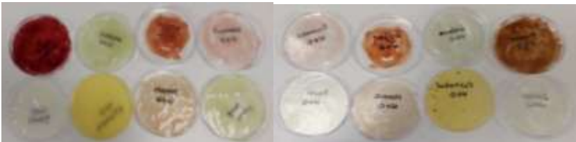
Figure 15. 10% Fresh fruit and vegetable waste and starch-added room-dried films
