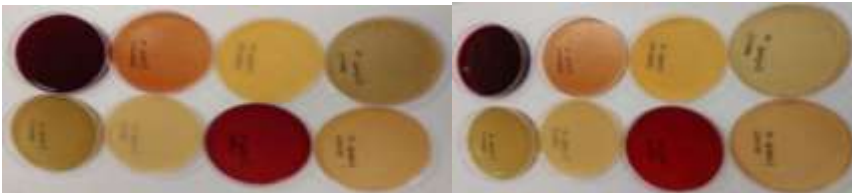
Figure 11. Microwave-dried fruit and vegetable waste and gelatin-added microwave + room-dried films
