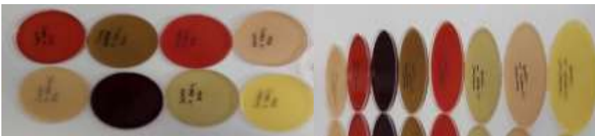
Figure 9. Oven-dried fruit and vegetable waste and gelatin-added room-dried films.
