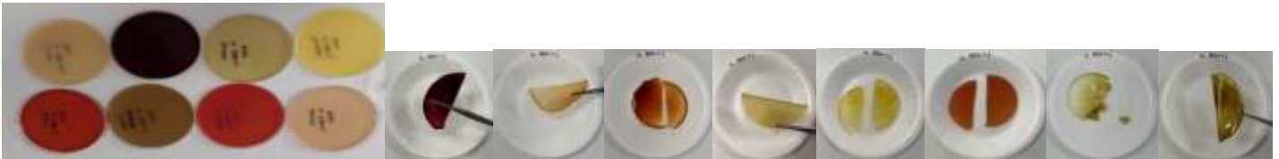
Figure 7. Oven-dried fruit and vegetable wastes and gelatin-added oven-dried films.
