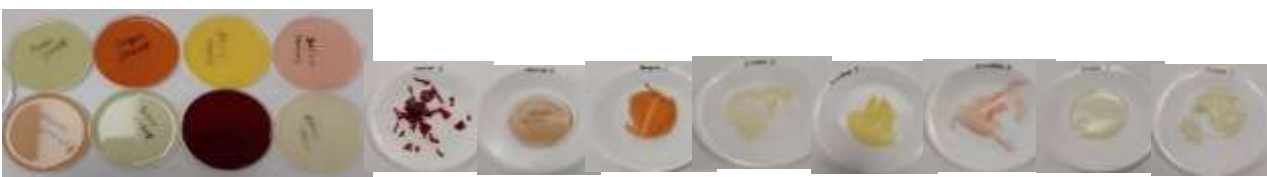
Figure. 25. 10% fresh fruit and vegetable wastes and added starch + gelatin in equal proportions and oven-dried films
