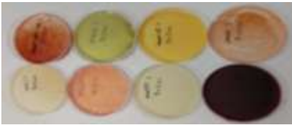
Figure 28. ½ Fresh fruit and vegetable waste and starch + gelatin added oven-dried films
