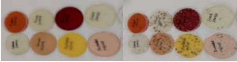
Figure. 27. 10% fresh fruit and vegetable wastes and added starch + gelatin in equal proportions and room-dried films
