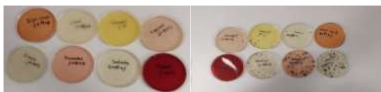
Figure 2. 10% fresh fruit and vegetable waste and gelatin-added films subjected to microwave + room drying
