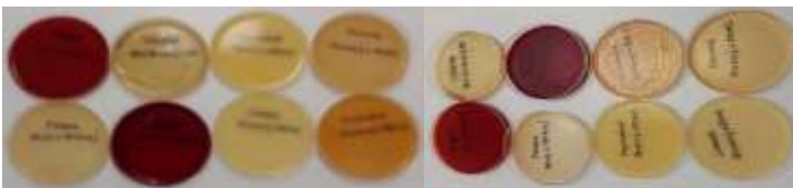
Figure 35. Microwave dried fruit and vegetable wastes and starch + gelatin added microwave + room-dried films
