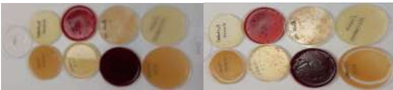
Figure 24. Microwave-dried fruit and vegetable wastes to which starch was added and room-dried films
