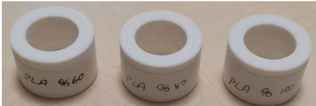
Fig. 2. Radial sliding bearings made of PLA at different filling ratio
