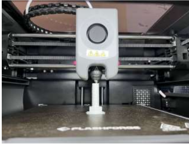
Figure 1. View at the moment of bolt printing with PLA material.
