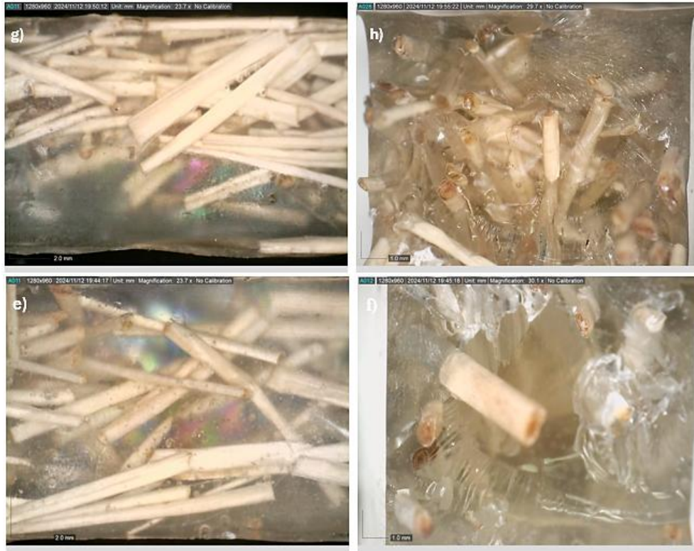
Figure 6. Microscopic images of epoxy matrix composites with 0%, 1%, 3%, and 5% banana fiber by weight
