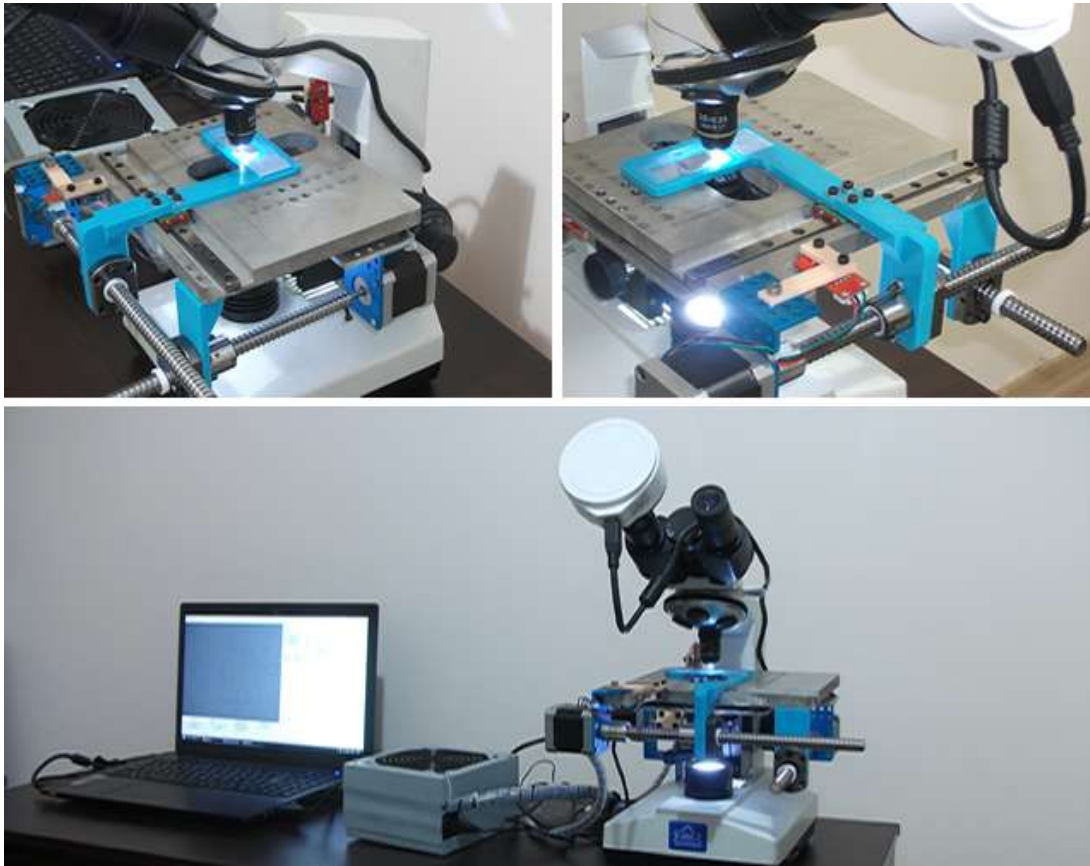
Fig. 5. Developed Motorized Microscope Stage.
