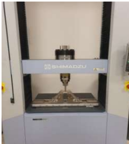
Figure 2. Three-point bending test setup
