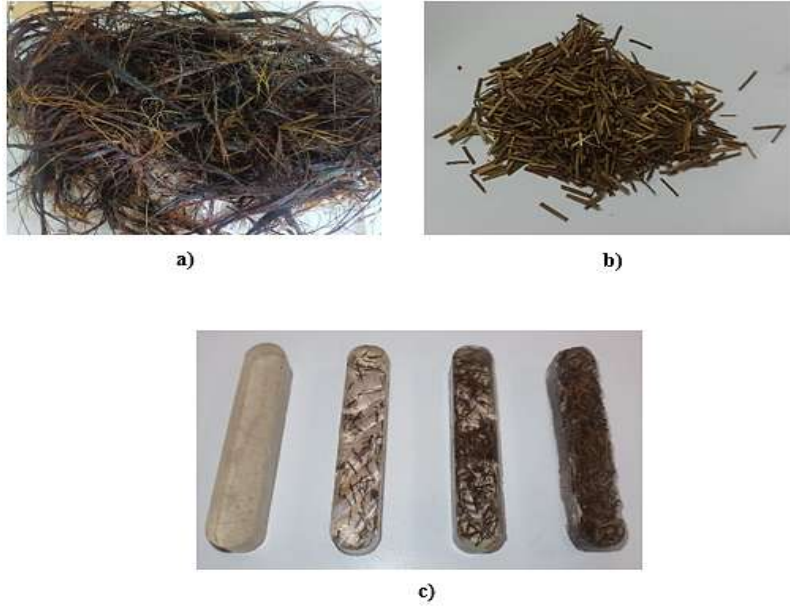
Figure 1. a) Surface-modified palm fibers, b) Chopped palm fibers, c) Three-point bending test specimens with palm fiber additions at weight ratios of 0%, 0.5%, 1.5%, and 3%
