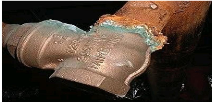
Fig 2. Schematic representation of Galvanic corrosion
