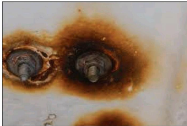
Fig 3. Schematic representation of crevice corrosion
