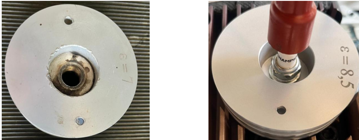
Fig. 2. the cylinder heads with varying CRs.
