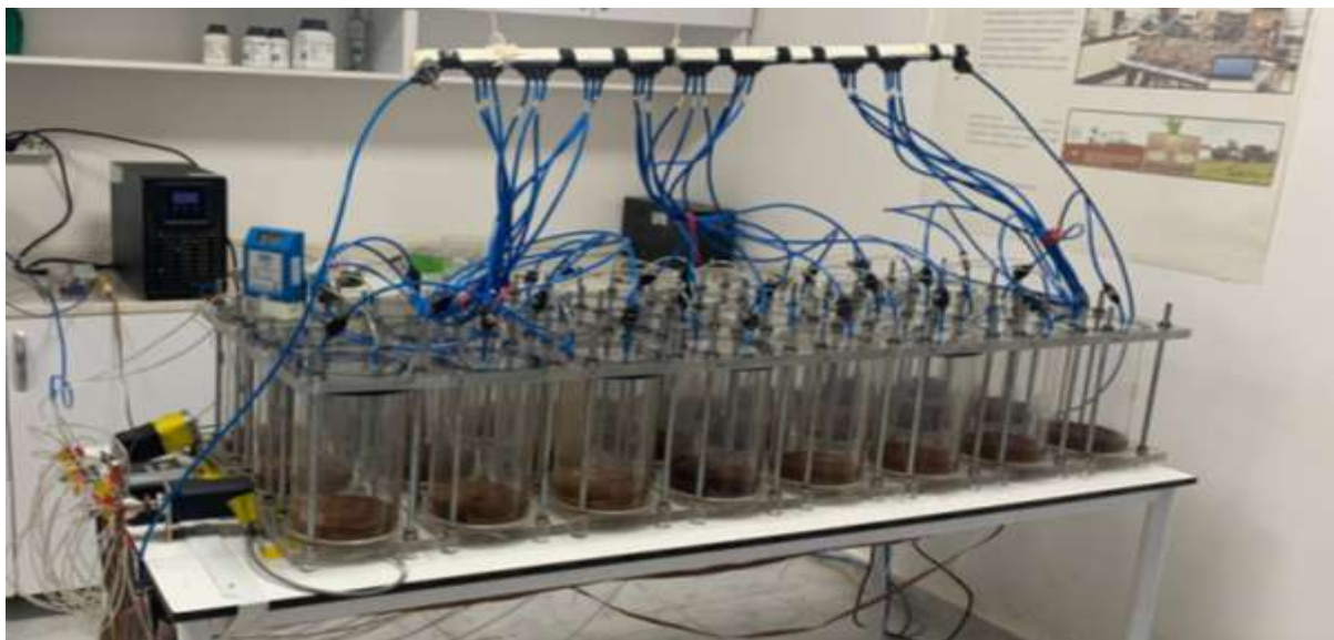
Figure 1. Continuous Flow Fully Automated Incubation System
