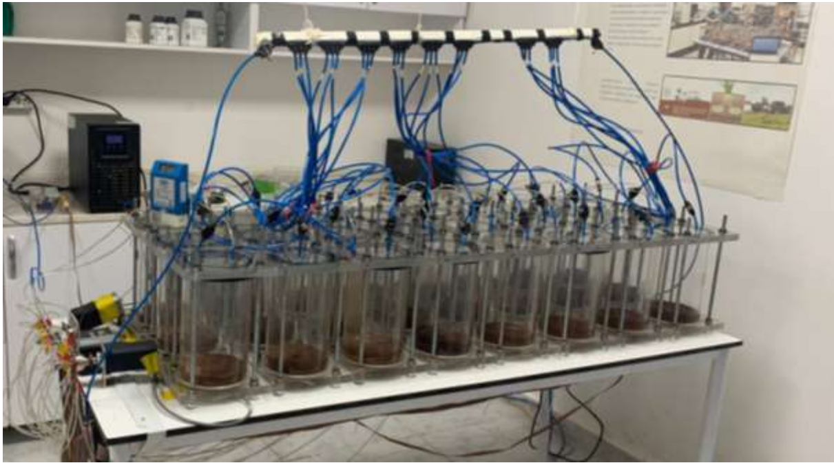
Figure 1. Continuous Flow Fully Automated Incubation System
