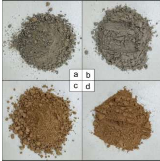
Figure 1. Raw natural pozzolan (a), milled pozzolan (b), raw clay (c), calcined milled clay (d)
