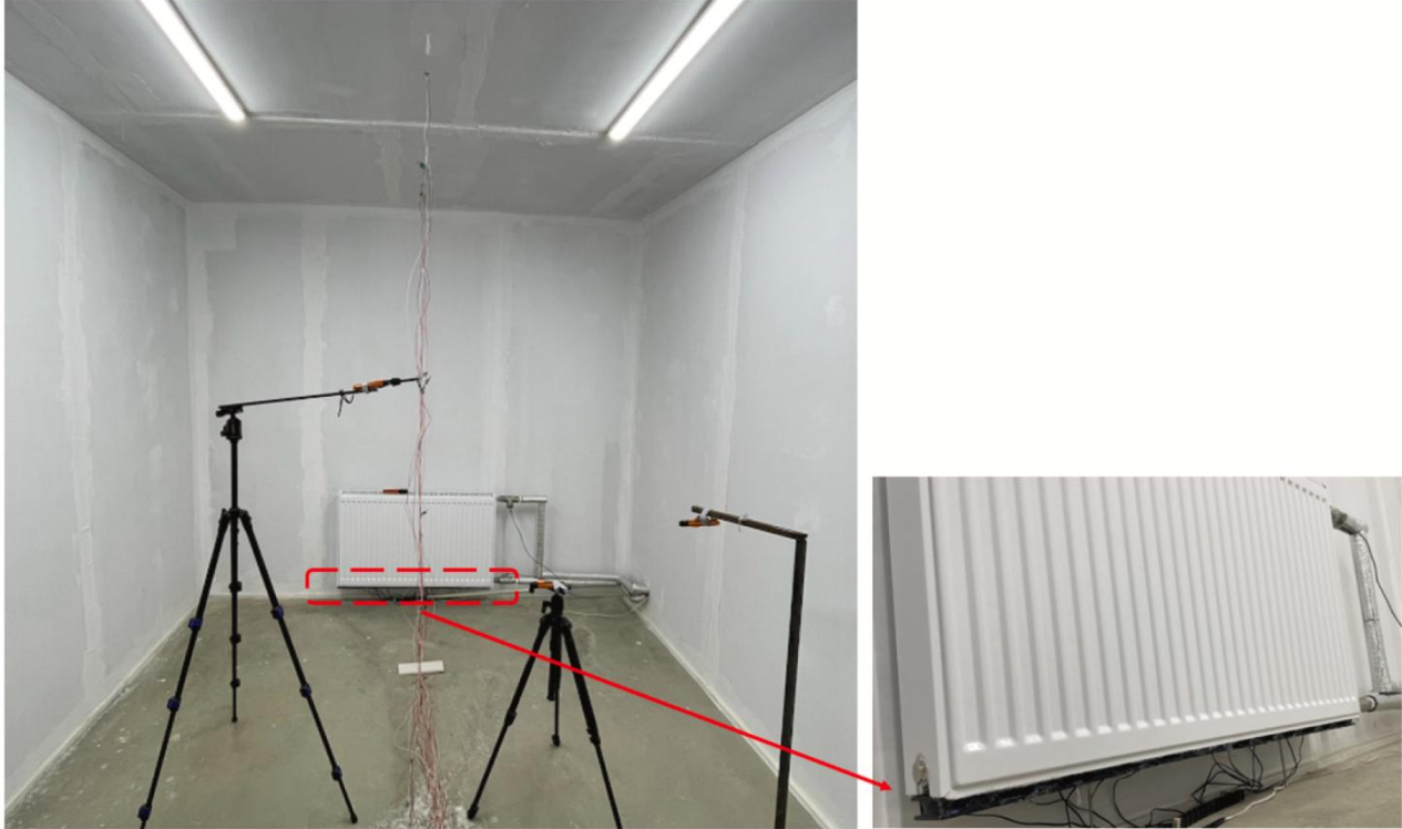
Figure 1. The test room and the add-on fan radiator
