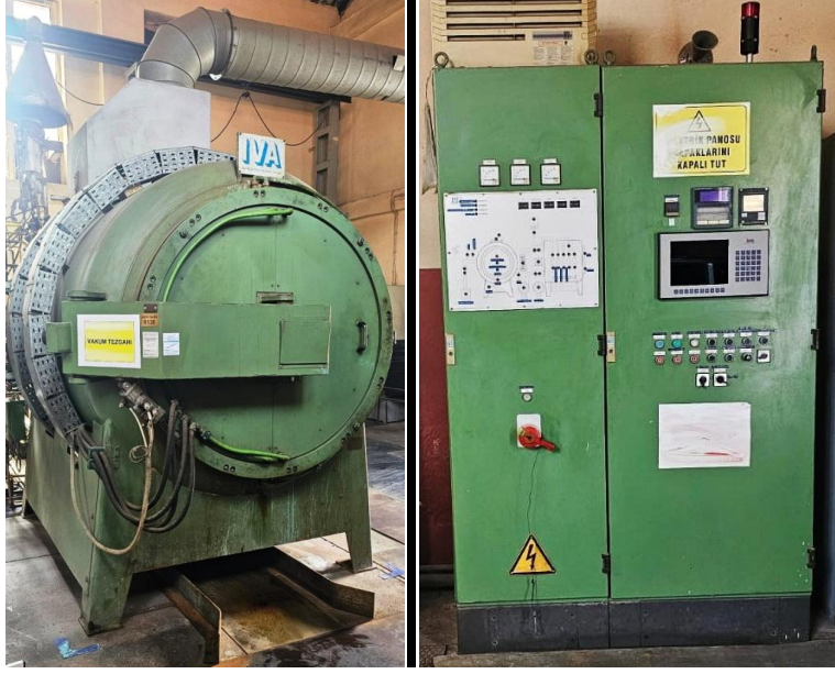
Figure 3. Gas nitration furnace and control board.
