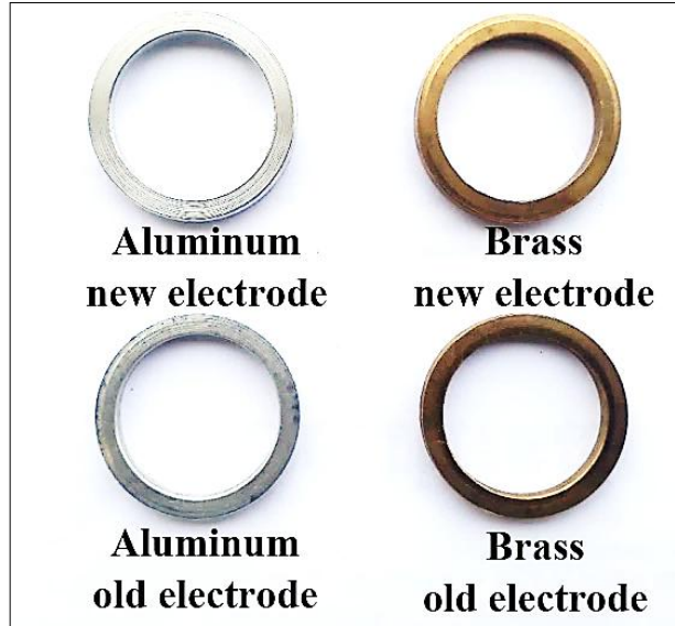
Figure 5: The electrodes used to investigate the effect of electrode age on charging efficiency.
