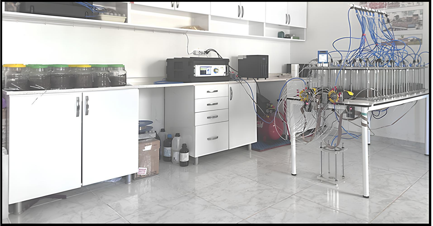
Figure 2. Robotic continuous-flow soil incubation system
