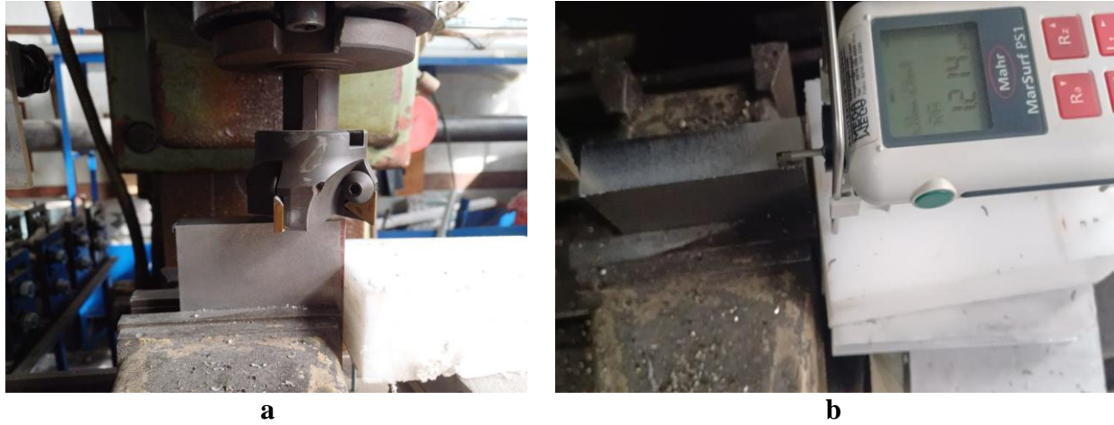
Figure 2. a) Milling process on universal milling machine, b) surface roughness measurement
