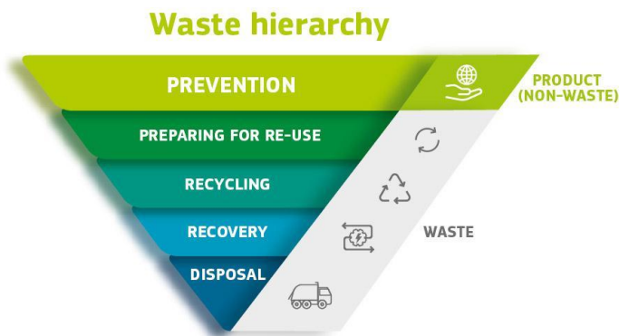
Figure 11 The waste hierarchy which is embodied in the EU Waste Framework Directive
