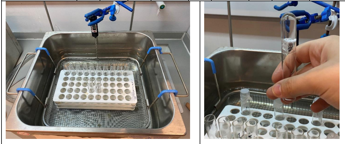
Figure 27. Sol-Gel temperature studies. The tubes were placed in the tube stands as seen in the left figure in which all the parts of tubes that have formulation made to touch water to get even heat from all directions. A digital thermometer (TP-Digital thermometer, India) was used to get exact temperature. After gelation, the tubes turned 90 and 180 degrees to check full gelation as seen in the right figure.
