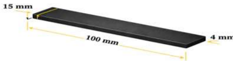
Figure 4: Composite specimen used for flexural strength tests.
