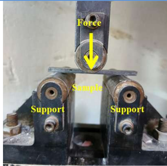
Figure 5: Experimental setup for the three-point bending test
