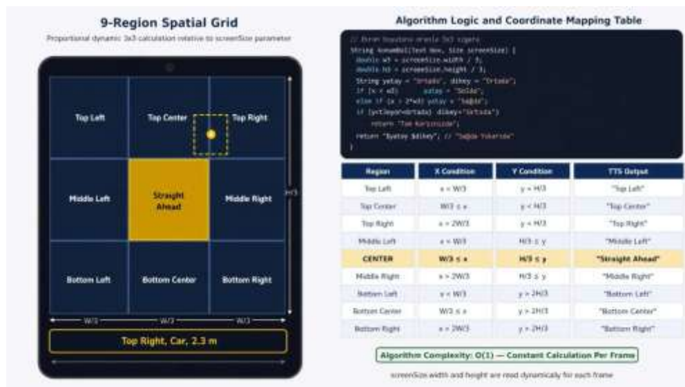
Figure 2. 9-region spatial grid — coordinate mapping algorithm and Turkish TTS output table
