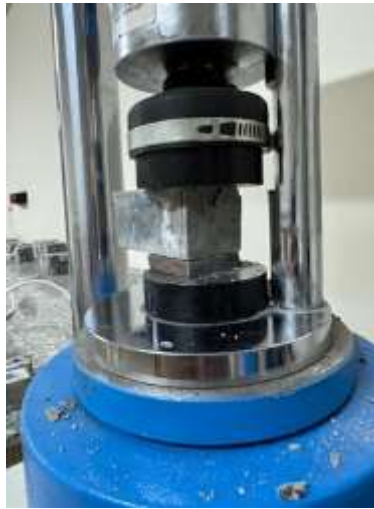
Figure 4. A compressive strength test setup conducted in accordance with the ASTM C349 (ASTM C349, 2013) standard.
