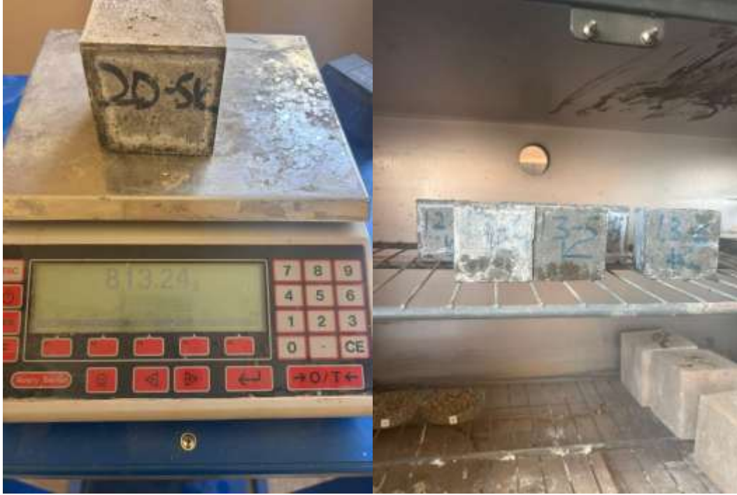
Figure 5. Images showing the oven-drying, immersion in water, and weighing of samples as part of a water absorption test.
