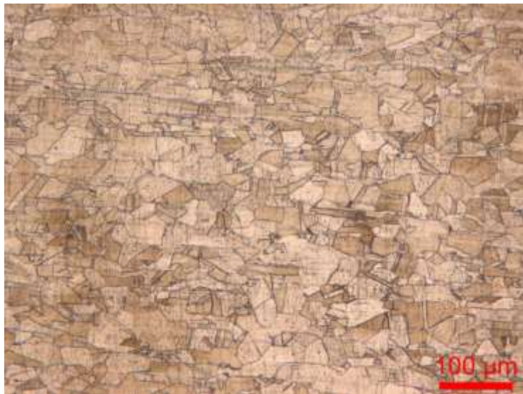
Figure 4. Microstructure of AISI 316L stainless steel alloy
