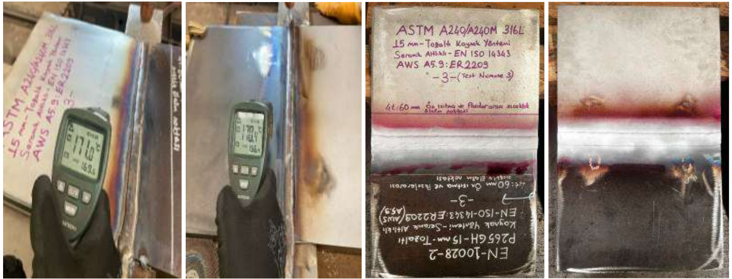
Figure 2. Submerged arc welded samples
