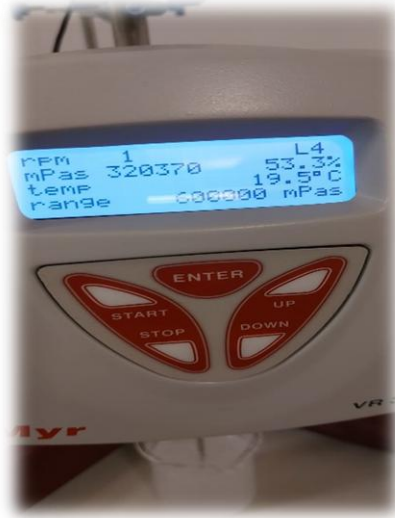
Figure 4. Viscometer device used to measure viscosity of optimum formulation.
