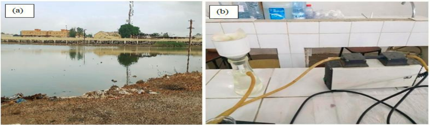
Figure 4. (a) Still water of the drilling site, (b) Installation of a Büchner filtration equipped with a 0.22\mu\text{m} pore size filter, University of Djibouti Laboratory (Original 2023)
