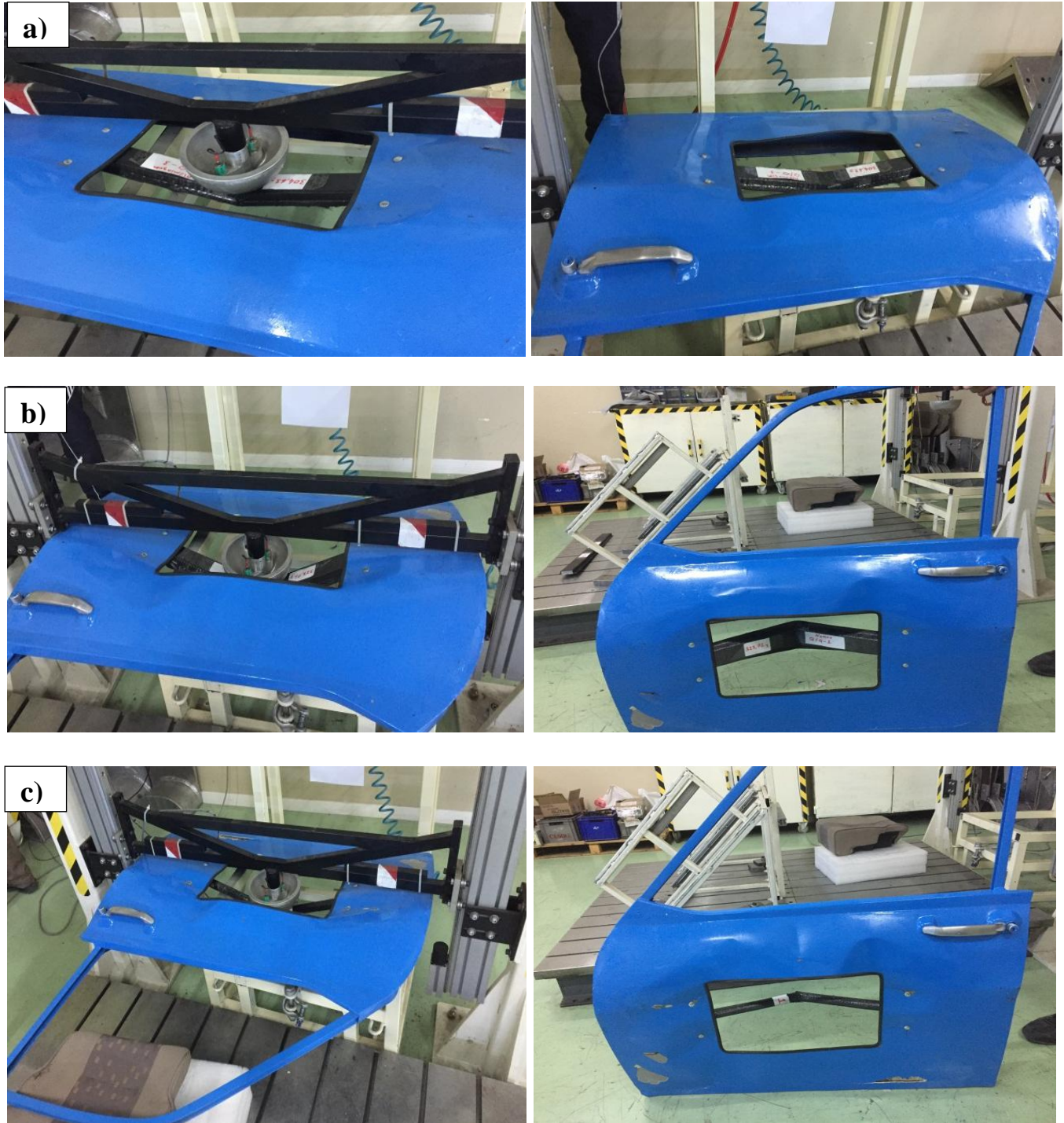
Figure 6. Free fall test a) Aluminum honeycomb carbon fiber material b) Nomex honeycomb carbon fiber material c) O profile carbon fiber material
