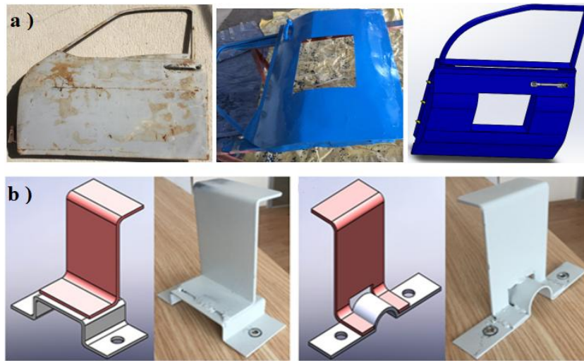
Figure 3. a) automobile door b) C profile and O profile clamp to be used in tests
