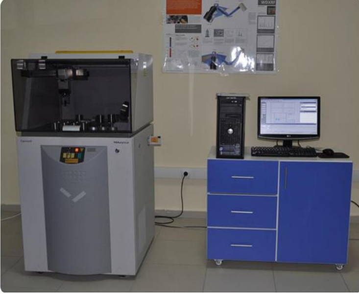
Figure 2. EDXRF (Energy Dispersive X-ray Fluorescence) spectrometer (Epsilon 5, PANalytical, Almelo, the Netherlands)
