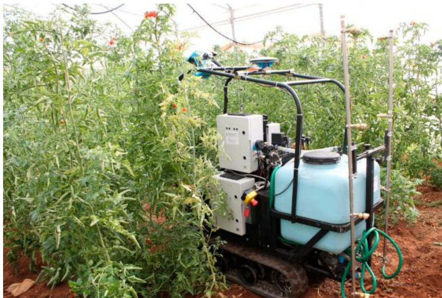
Figure 4. The developed spraying robot while operating in a greenhouse (Cantelli et al., 2019).
