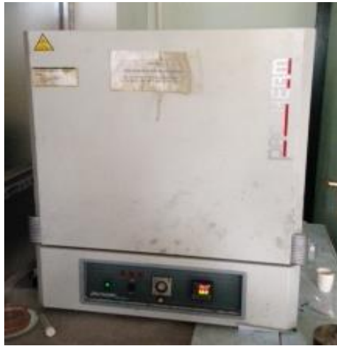
Fig. 2. Protherm brand furnace used in the foaming process.
