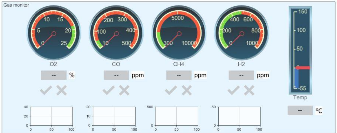
Fig. 3: Real-time gas monitor.
