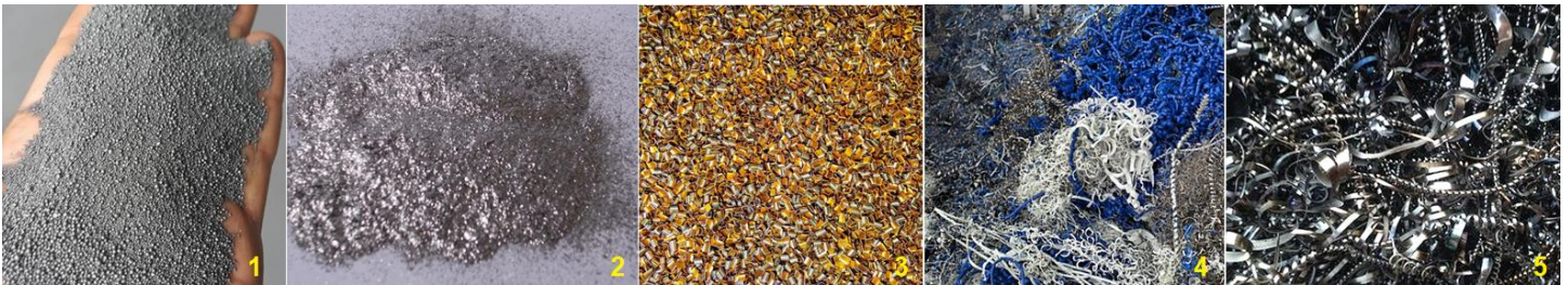
Figure 2. Recycle parts(1:Iron, 2:Aluminium, 3: Brass, 4:Plastic, 5:Steel)
