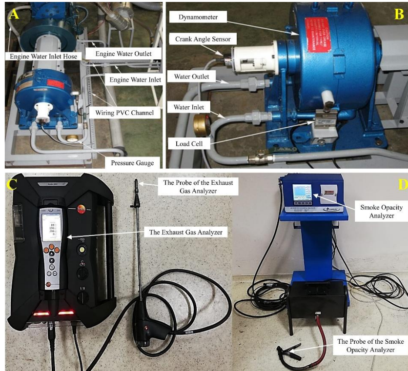
Figure 3. Engine Test Setup and Exhaust Gas Analysis Devices
