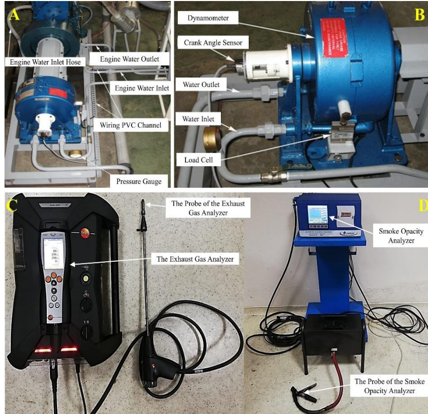
Figure 3. Engine Test Setup and Exhaust Gas Analysis Devices
