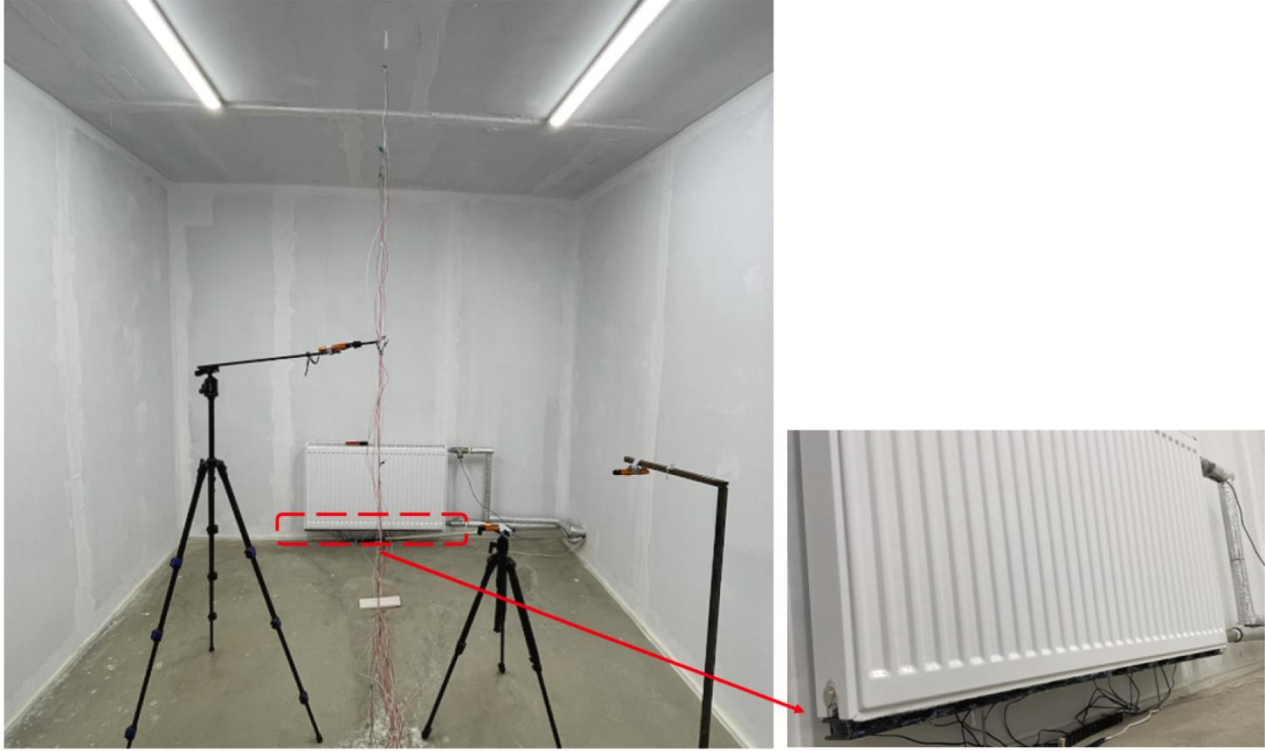
Figure 1. The test room and the add-on fan radiator
